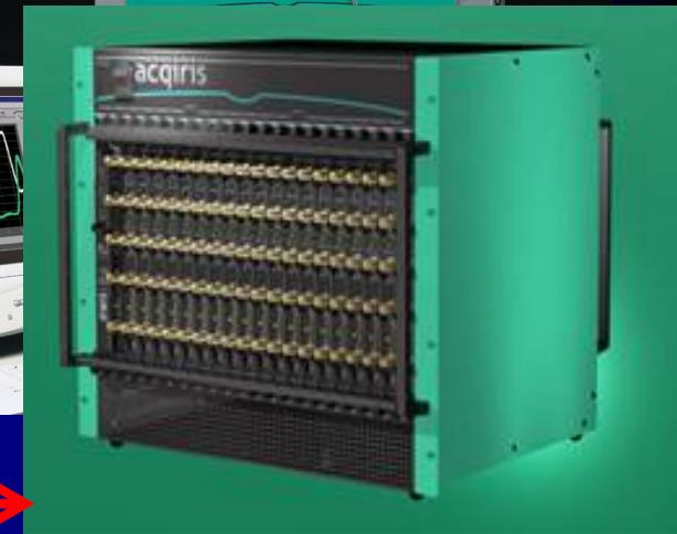
Digital Signal Processing Backend 18×1 GHz, 16384 pts each
