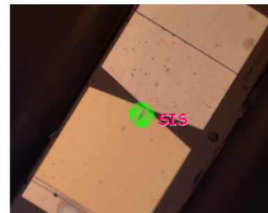
Photo of an NbN SIS junction (designed at PMO, fabricated at NiCT)
