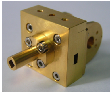
Photo of the 1st band-10 waveguide mixer block (designed/ordered by PMO)
